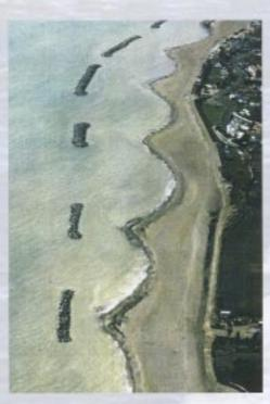
The Southern coast of England is characterised by rock outcrops and relevant tide excursion. ELMER presents a beach renourishment with shore parallel breakwaters to reduce wave energy and modify the nearshore wave climate.
