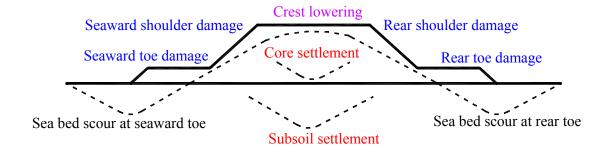
Please insert a sketch with dimensions of LCS cross-section when it was build compared to the appearance now (like the figure of failure modes) if possible.
