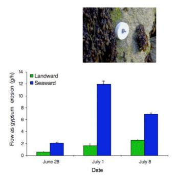
Fig. 1. Erosion of gypsum as a measure of average water motion. The photo inset shows a discs gypsum disc attached to an LCS in Elmer, UK. The graph shows the difference in erosion rates between the landward and the seaward side for 3 dates.
