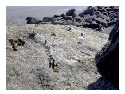
Fig. 2. Drag probes used to record maximum drag forces. For standardised measurements, allowing conversion to flow speeds, a training golf ball is used as a bluff body. The technique also allows the recording of maximum drag forces operating on individuals of *Fucus vesiculosus*.
