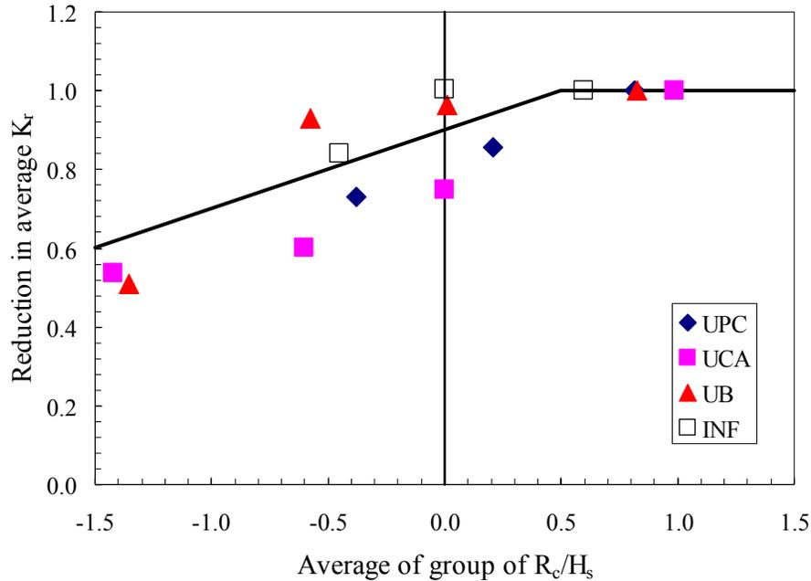
**Figure 9.** Reduction in reflection coefficient for low-crested rubble mound structures
