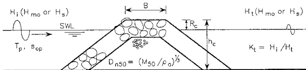
**Figure 1.** Governing parameters for wave transmission
