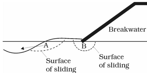
**Figure 12 Possibility of sand slide in front of breakwater.**
