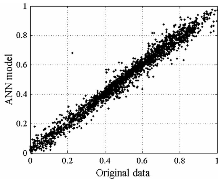
**Figure 5.** Comparison of wave transmission predicted by the neural network and measured
