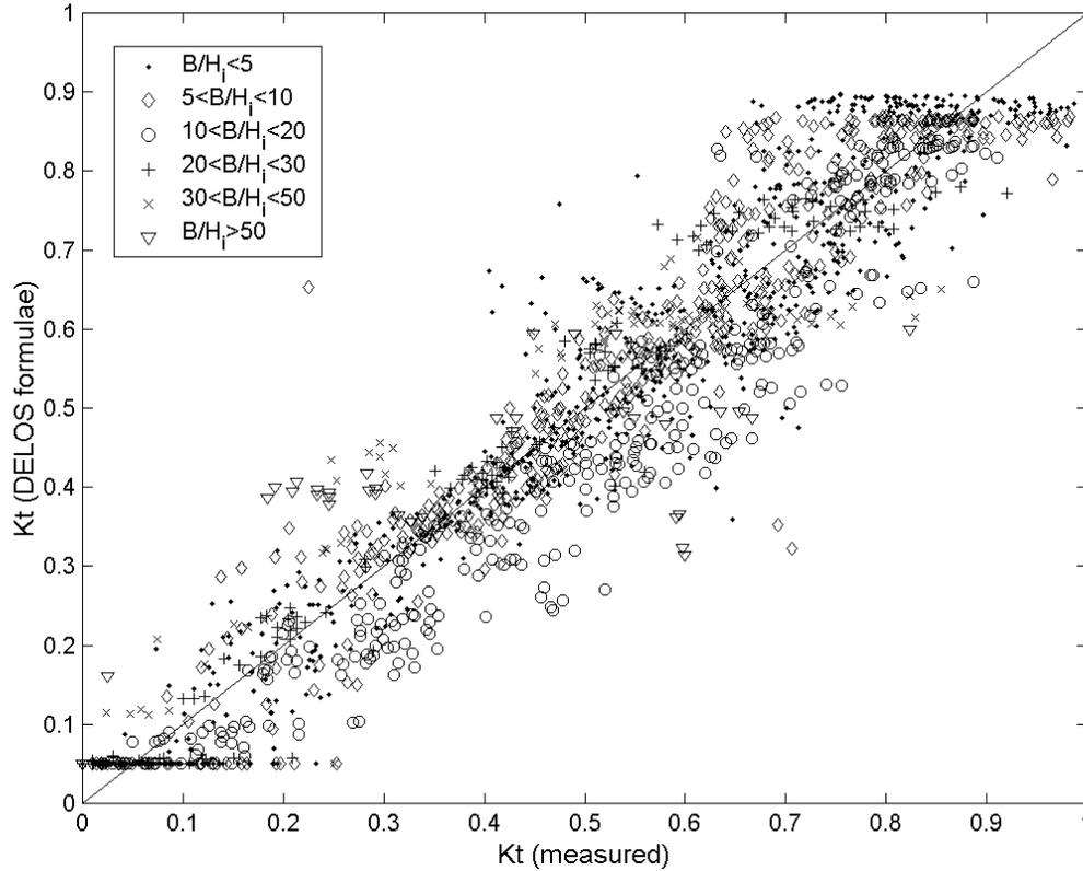
**Figure 2.** Calculated and measured transmission coefficients on rubble mound structures (Briganti et al. 2003)
