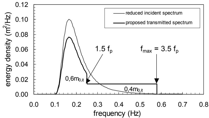
**Figure 7.** Proposed method by Van der Meer et al. (2000) for transmitted spectrum
