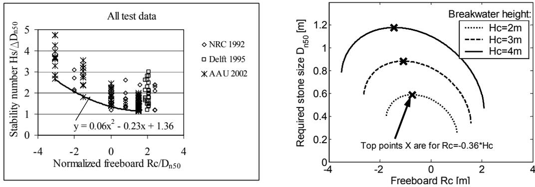
Figure 10. Design graphs for stability of low crested breakwaters corresponding to initiation of damage. Test results (left) and formula in case of depth limited waves (right).
