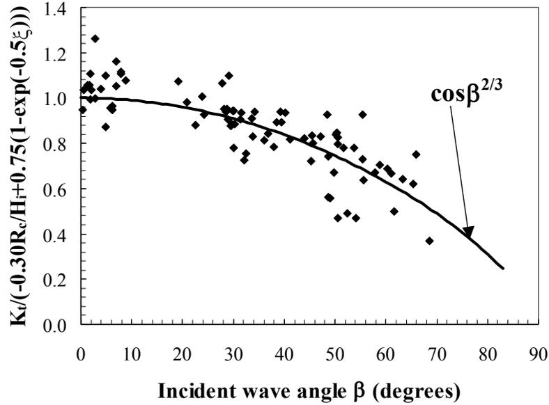
**Figure 3.** Influence of angle of wave attack on wave transmission for smooth structures
