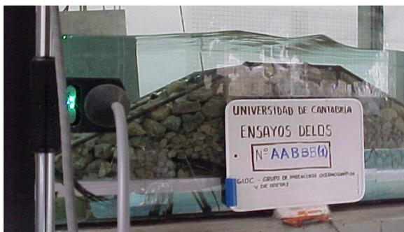
**Photo 7. LDA measuring in the front slope of the LCS. The square grid for the video camera is also shown attached to the flume glass.**
