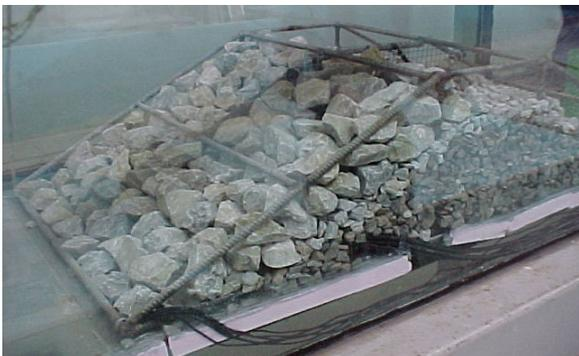
**Photo 3. ADPs just protruding from the surface of the LCS armour.**
