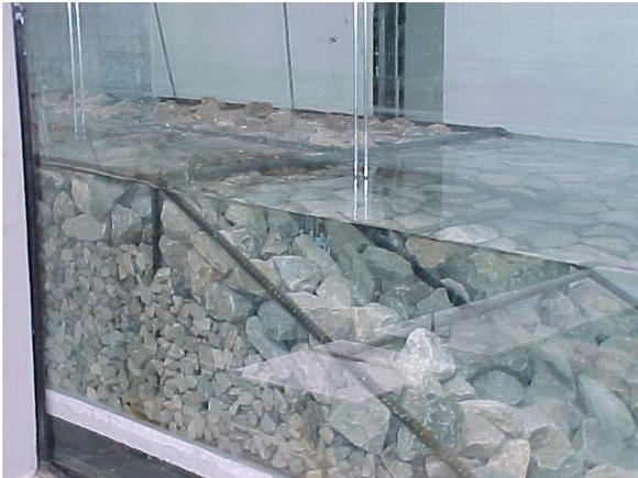
**Photo 9. Free surface gauges over the structure for the 1.0-m crest width.**
