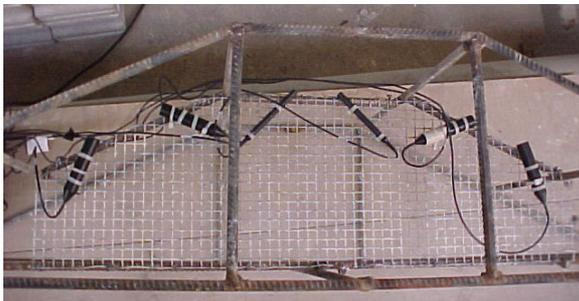
**Photo 2. ADPs attached to the steel frame before laying the core and armour stones.**
