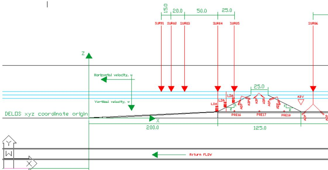
**Figure 2. Coordinate system, instruments and measurement points in front of the LCS**
