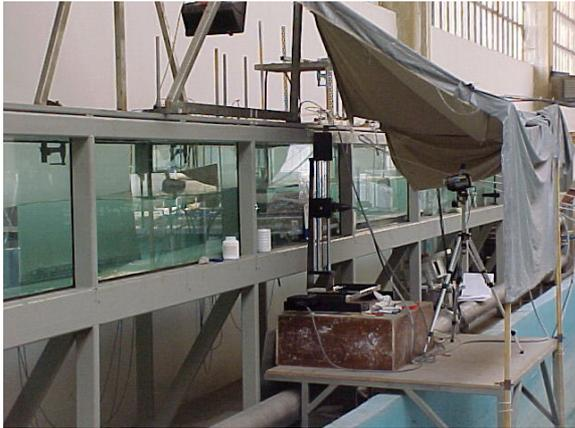
**Photo 8. LDA traversing system and video camera.**
