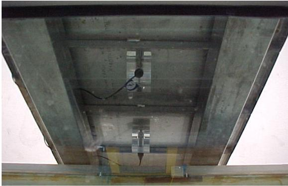
**Photo 4. ADPs attached to the steel false bottom to be installed horizontally in the transmission zone. Photograph from below the plate**
