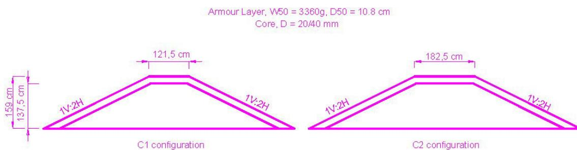
**Figure 26. Tested LCS sections.**
