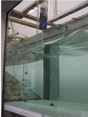
**Photo 1. ADV measuring behind the LCS back slope.**
