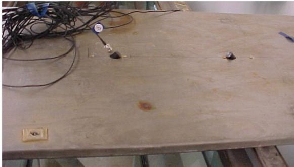
**Photo 5. ADPs attached to the steel false bottom to be installed horizontally in the transmission zone. Photograph from above the plate.**
