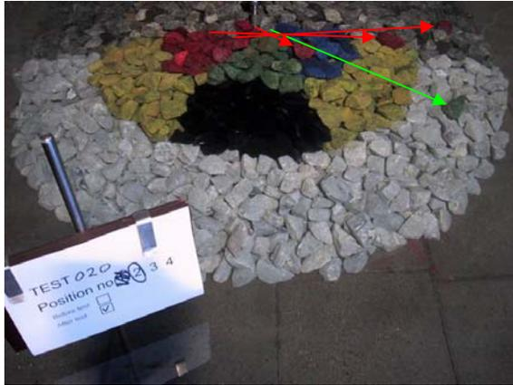
Figure 14 Tracking the stone movements
