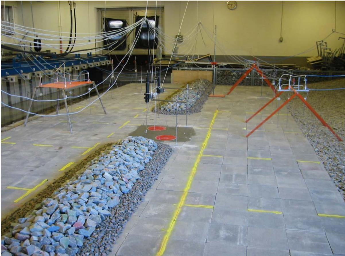
Fig. 2.3 Layout 1, side view of the instrumented basin, narrow berm.
