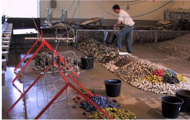
The basin was filled with water such that the water depth was equal to target zero freeboard. The crest height was then given a final adjustment by moving and adding stones such that a precise freeboard was obtained.
